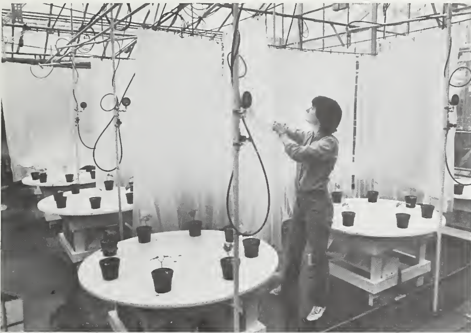
Acid rain's about to fall on test plants. Gwyn Trueblood adjusts curtains to keep plants from being splashed by neighboring showers. Tabletops rotate to ensure equal doses during simulation. (0986X1056-30)
